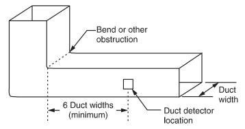
Duct detectors continually sample air flow in a HVAC duct and initiate an alarm condition whenever smoke is detected. An alarm is activated when the quantity (percent obscuration) of combustion products in that air sample exceeds the detector's sensitivity setting.
